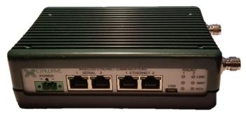
also be used to bridge between two different frequency bands or bridge between two networks. **Compatibility** with **MDS x710**, **SD Series**, and **TransNET**<sup>TM</sup> master and repeater radios is supported and the **Dual Band** radio also supports full duplex operation.
